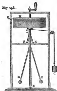
FIG. 198. YOUNG'S METHOD OF RECORDING MINUTE INTERVALS OF TIME BY MEANS OF A VIBRATING STYLE WRITING ON A REVOLVING CYLINDER.
